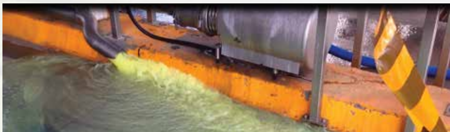
Visual example of losses of whey & permeate from the Tanker Bay draining to Trade Waste System.
